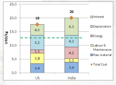
Figure 2: Cost Break-up of Polysilicon Manufacturing
